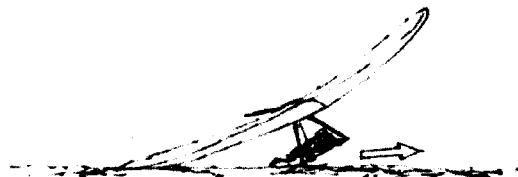
④ PILOT AND BASE TUBE SLIDES SIDEWAYS IF GLIDER DOESN'T TURN ALL THE WAY AROUND INTO THE WIND.
